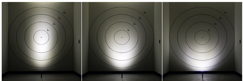
Mini LED Spotlight Beam Patterns: 15° (left), 30°, 60°
